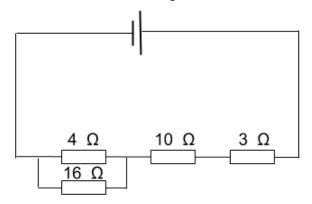
Firstly, find the resistance of the parallel combinations of resistors:
