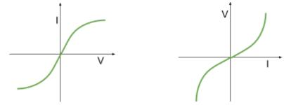
(Negative Temperature Coefficient) Thermistor - This component acts in the opposite way
